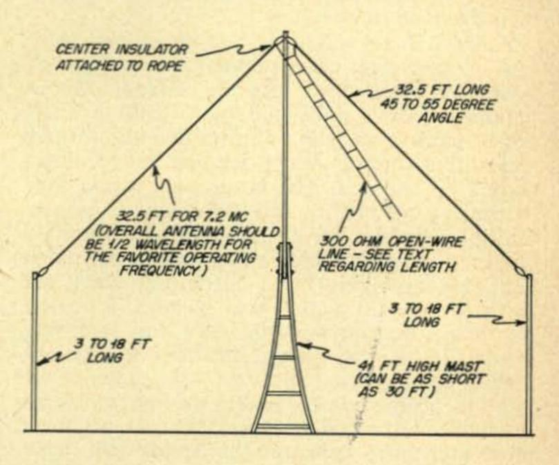
Each quarter-wave leg droops down at a 45 to 55 degree angle and the ends may be supported near the ground by any available support, from three to 12 feet high, depending upon the height of the center mast and the angle of descent of the legs of the antenna. Number 12 wire is used, but for a time we tried number 24 and it worked just as well!
